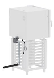
The drain box can be mounted with the outlet to the left or to the right as required by the installer (just unscrew the drain box cover and turn the assembly 180° and screw it back on).
